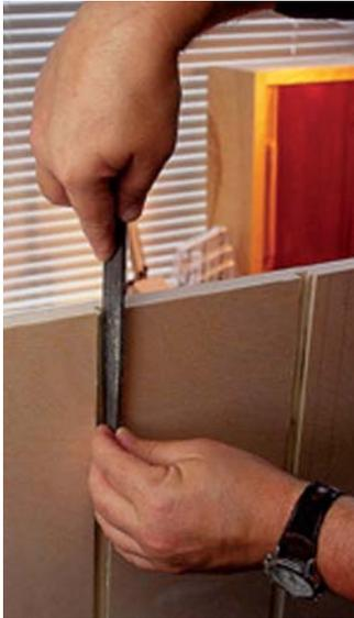
The veneer edge tape is easy to use and quickly adds a finished appearance to the cabinet. Even though we ended up painting the exterior, the paint still applied better to the veneer tape than on a bare plywood edge. You'll need to notch the tape with a file at the dado locations in the left case side.
