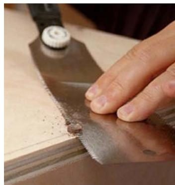
Before attaching the second side, it makes sense to cut the dowels on the first side flush to the surface. I used a Japanese flush-cutting pull saw that has teeth with very little set to them, reducing the chance of scratching the cabinet side. By applying pressure on the blade to keep it flat to the cabinet surface, I further reduced the chance of scratches. Do a little sanding, then flip the cabinet over and attach the second side, then the front.
