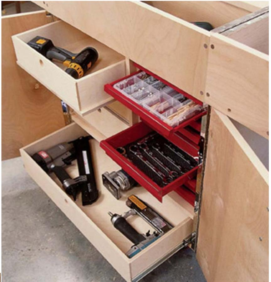
Pads line the bottoms of the wing and till sections to keep tools from rolling and to help trap dust. Dividers in the till section can be customized to fit the tools you need. The magnetic bars on the till lid provide secure storage for small ferrous tools. Small-parts storage is easily accomplished with a couple of plastic storage bins held in place in one of the metal drawers with some hook-and-loop fasteners.
